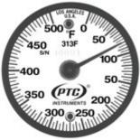
relatively quick response time. The thermometer reaches sensing equilibrium (stability) within three minutes. Single or max-min ancillary hands are available for this instrument as an option.
