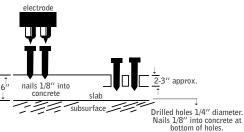
If the meter still indicates green or "dry," the floor should be ready for covering. Tests should only be made in newly drilled holes, since the inside surface of the holes can dry out while the rest of the slab is still wet.
