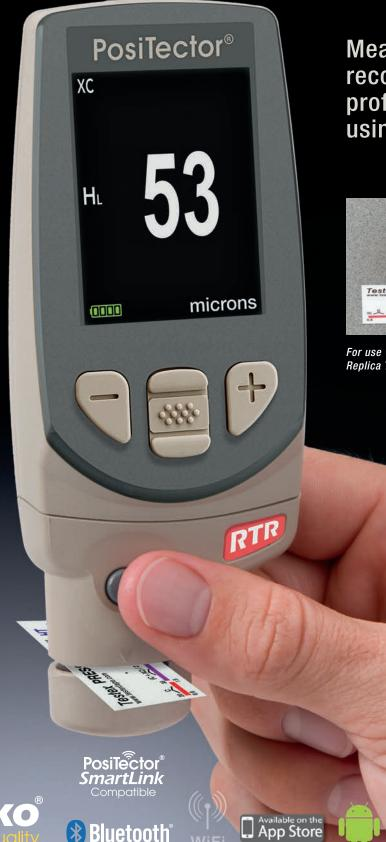
Measures and records surface profile parameters using replica tape
